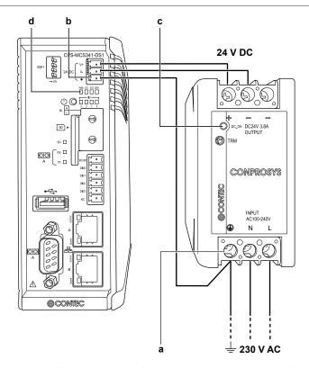
1 Connect the power supply to the 3 terminals, L (live), N (neutral) and ground in the input section of the power supply (PS).
