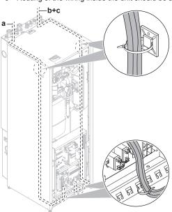
4 Fix the cable with cable ties to the cable tie mountings to ensure strain relief and to make sure that it does NOT come in contact with the piping and sharp edges.
