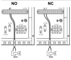
2 Fix the cable with cable ties to the cable tie mountings.
