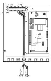
2 Fix the cable with cable ties to the cable tie mountings.
