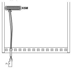
4 Fix the cable with cable ties to the cable tie mountings.
