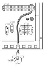
2 Fix the cable with cable ties to the cable tie mountings.
