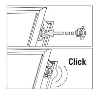
Fig. 3-28 Insert the end plugs
