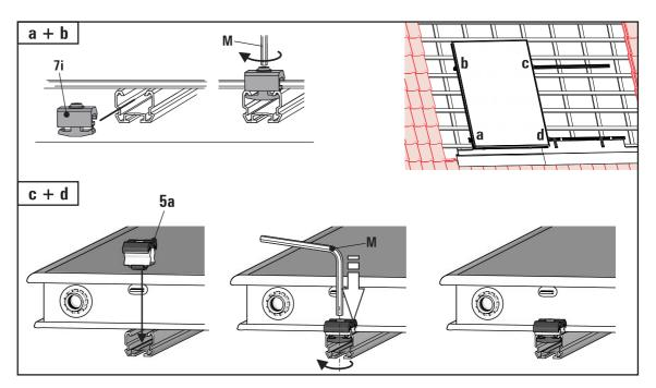
Fig. 3-19 Screw flat solar panel with individual single clamping blocks (7i) on the mounting profile rails and insert double clamping blocks (5a).
