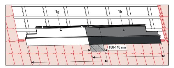
Fig. 3-15 Ensure that the respective covering sheets (1g / 1h) interlock and overlap sufficiently from both sides.
