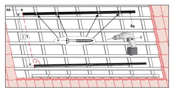
Fig. 3-11 Set up upper mounting rails (4a) parallel to the lower mounting rails and fix with particle board screws (H) on the rafters.
