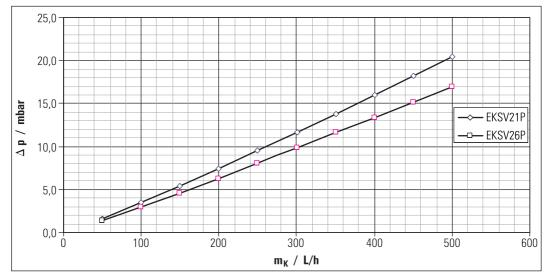
Fig. 5-1 Hydraulic resistance flat solar panels
