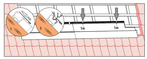
Fig. 3-16 Fix right covering sheet (1h) (same procedure like left covering sheet (1g)).
