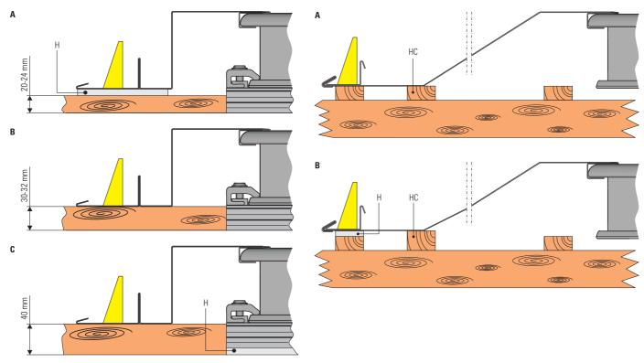
Fig. 3-4 Auxiliary strips mounted on the side part depending on the roof batten thickness (Key see fig. 3-3)
