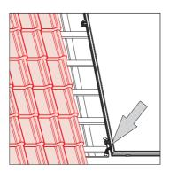
Fig. 3-36 Installation position for collector temperature sensor - p=0
