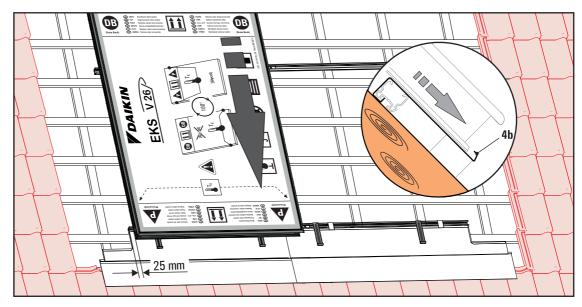
Fig. 3-18 Lift the flat solar panel over the mounting rails, and carefully suspend it in the solar panel securing hooks (4b).
