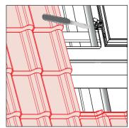
Lead through the connection pipe below the solar panel field
