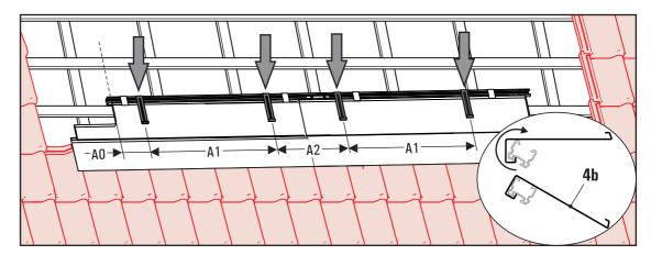
Fig. 3-17 Hang solar panel securing hooks (4b) into the upper side guiding groove of the lower mounting rails and tilt downwards.
