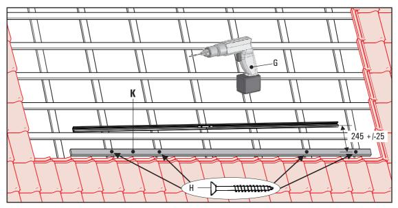
Fig. 3-10 Fix lower auxiliary batten (K) with particle board screws (H) in the specified distance to the mounting rails.
