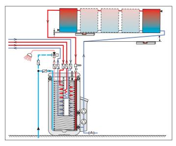
Fig. 3-1 Solar system solar panels connected at opposite ends with hot water storage tank EKHWP\* (shown on drain-back system P=0 ).
