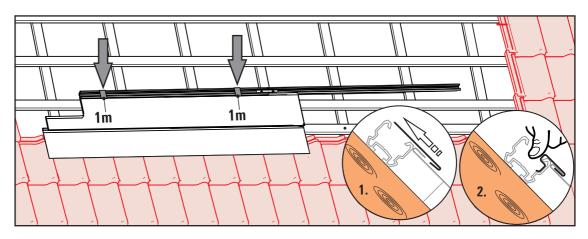
Fig. 3-14 Fix left covering sheet (1g) with safety sheets (1m) (hook it from below into the covering plate and then bend inwardly into the mounting profile edge).
