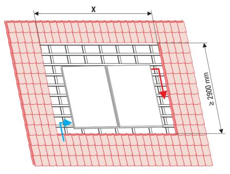
Fig. 3-8 Cover roof area (Dimension X = Dimension C in tab. 3-3)
