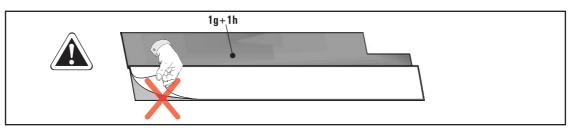
Fig. 3-12 Mount all of the flat solar panels before removing the covering foil for the bitumen strip during the covering process (section 3.4.9)!
