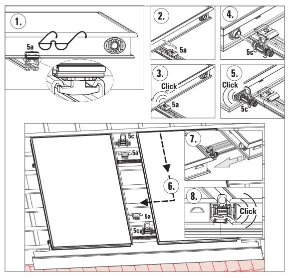
Fig. 3-20 Install double clamping blocks (5a) and expansion joints (5c). Installing flat solar panel in case of big solar panel fields, install additional solar panels in same procedure.
