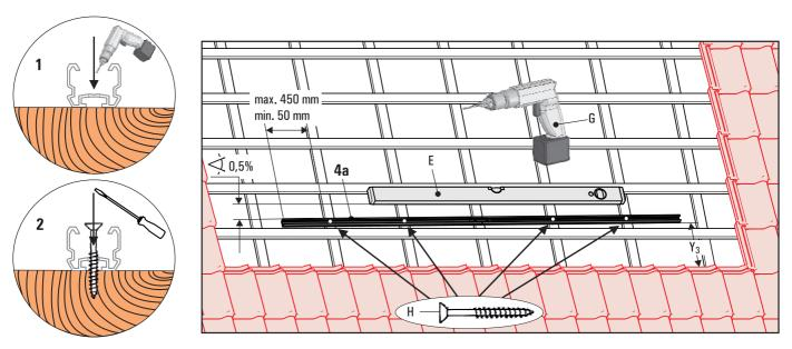
Fig. 3-9 Adjust lower mounting rails (4a) and tighten with particle board screws (H) on the rafters.
