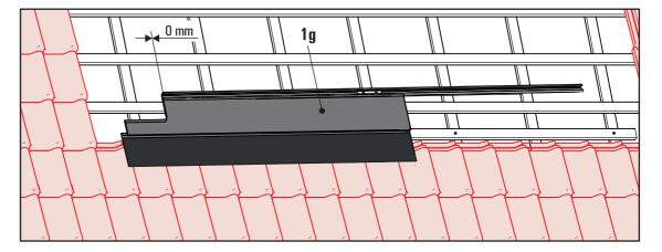
Fig. 3-13 Erect left covering sheet (1g) distance on the mounting profile rails.
