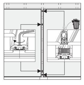
Fig. 3-21 Tighten double clamping blocks between the flat solar panels and detach assembly supports from the expansion joints.
