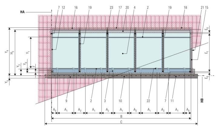
Fig. 3-2 Main dimensions of a Solar system solar panel with Solar collectors in-roof mounting (shown on the flat solar panel EKSV26P in the drain-back system)
