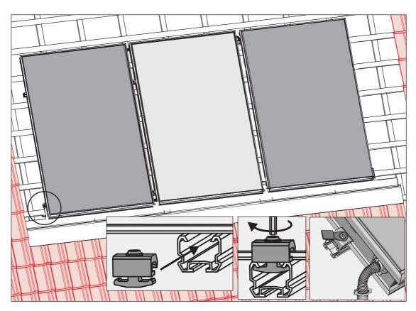
Fig. 3-22 Insert the individual clamping blocks for the last flat solar panel and tighten down. Mount the clamping block with potential balancing terminal close to the return flow connection. Shown on a flat solar panel EKSV26P in drain-back system
